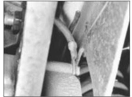
7C.33 Disconnect the transmission earth strap
