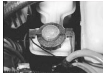
14B.54 Master cylinder/vacuum servo located next to the coolant expansion tank (1301 cc Turbo ie model)
