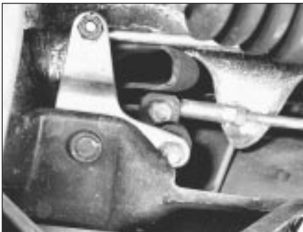
12B.31 Gear control and selector link rod joints
