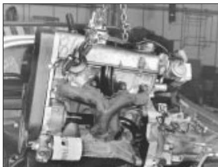
5C.34 Lifting out the engine and transmission
