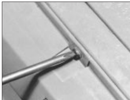
17.22 Radiator grille screw removal on a 1372 cc SX ie model
