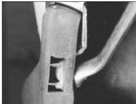
17.29 Unscrewing a bumper end fixing nut
