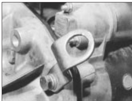
5D.38 Lifting eye on flywheel housing flange
