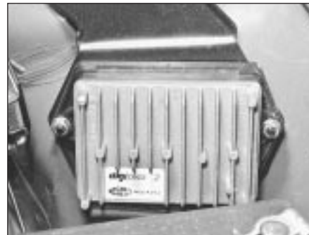
10.68 ECU location on the 1372 cc ie engine
