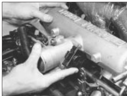
9C.73 Removing the inlet manifold
