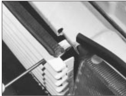
17.19B Prising down a radiator grille clip
