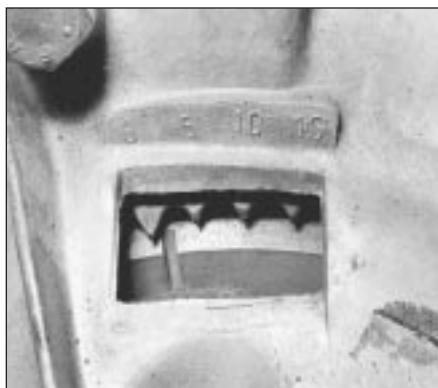
10.2A Flywheel timing marks (999 cc engine)
