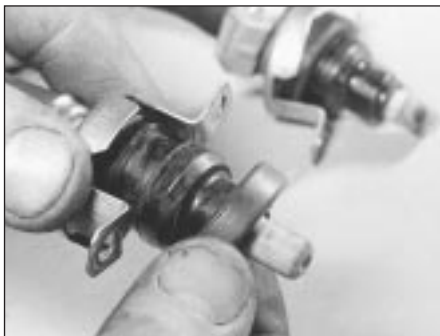
9C.95A Fuel injector large seal
