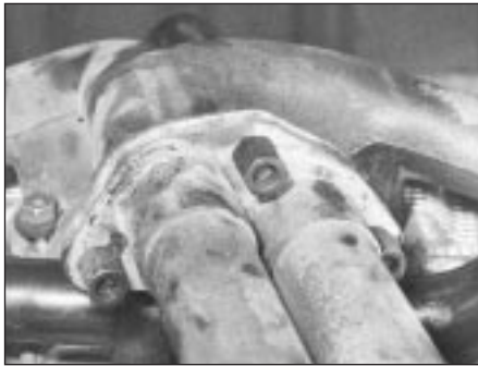
5C.23A Exhaust downpipe flange nuts
