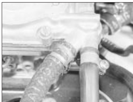
9B.37A Fuel inlet and return hoses on the Weber 30/32 DMTE carburettor
