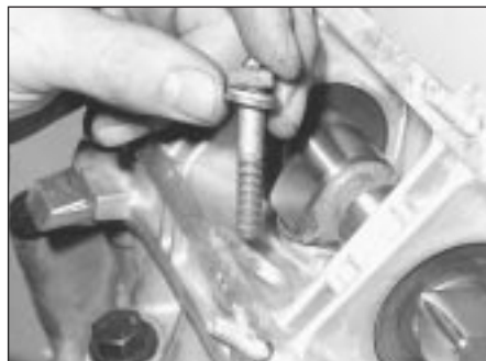
7B.77 Removing one of the camshaft housing shorter securing bolts
