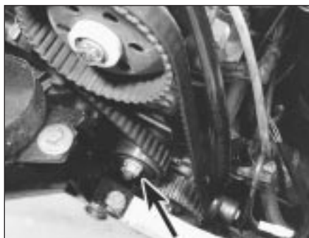
6B.20 Belt tensioner pulley locknut (arrowed)
