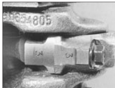
5B.88 Connecting rod and cap numbers
