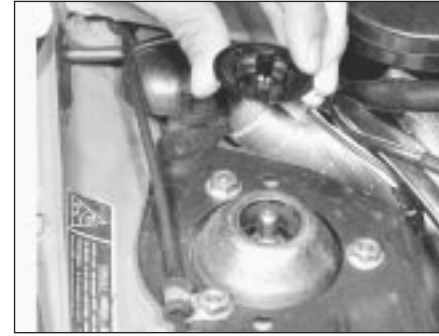
16.7 Suspension strut upper mounting nuts, showing bracket and cable clip on the 1372 cc ie model
