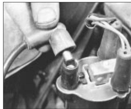
5C.15 Ignition coil HT lead connection
