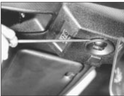
15.82 Roof-mounted clock retaining screw removal
