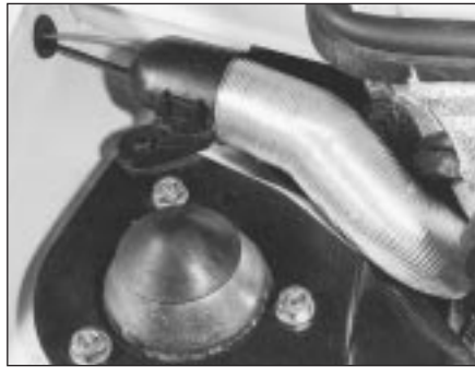
15.12A Alternator air cooling hose
