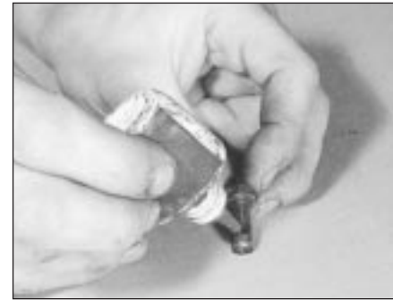
14B.10 Applying thread-locking fluid to the bolt threads
