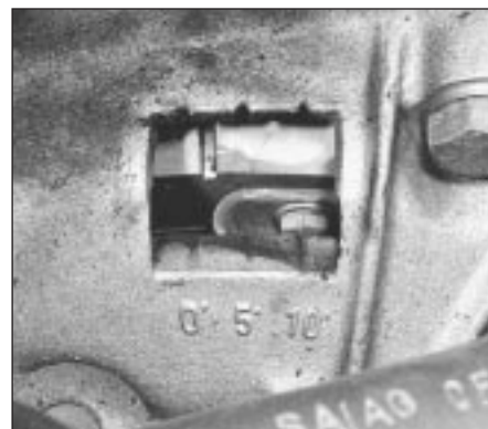
10.2B Flywheel timing marks (1372 cc ie engine)
