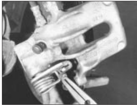
14B.36 Disconnecting the handbrake cable from the caliper lever
