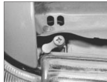
15.31B Headlamp vertical beam alignment adjuster screw on a 1372 cc ie model. Note the load compensator lever which is set in the "O" (normal load) setting position
