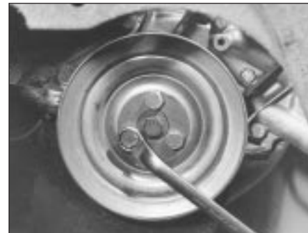
5B.7 Unscrewing the crankshaft pulley bolts
