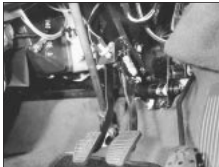
14B.47 Right-hand end of brake pedal cross-shaft
