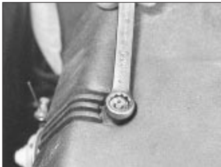
9A.6 Air cleaner casing nut on the 999 cc model
