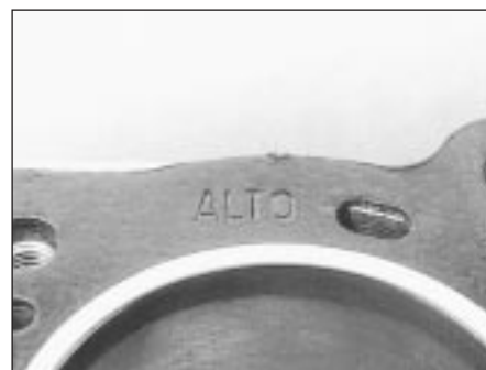
5B.50B Cylinder head gasket top surface marking
