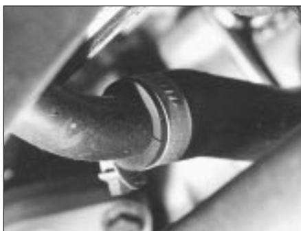
9F.20 Turbocharger oil return pipe at sump
