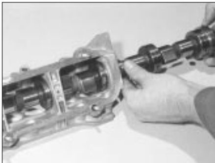
7B.93 Withdrawing the camshaft from its housing
