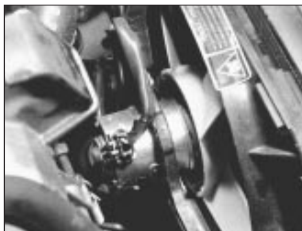
8C.21A Cooling fan and wiring connector
