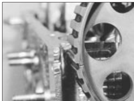
5B.8A Camshaft sprocket timing mark and cylinder head timing mark in alignment
