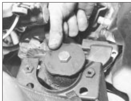
5C.31A Right-hand engine mounting disconnected
