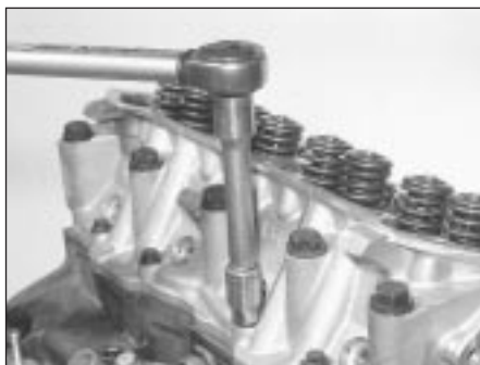
7B.122 Tighten the smaller cylinder head bolts to their specified torque setting
