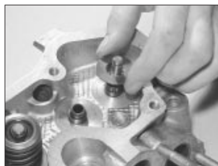
7B.130E Refit the flat washer . . .
