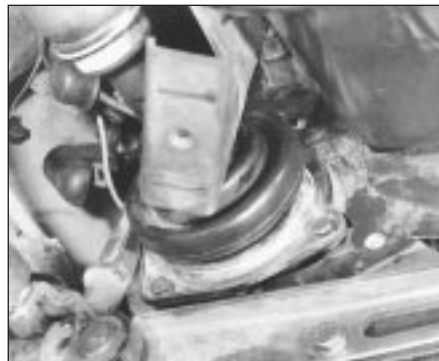
5C.24C Gearchange rod support bracket
