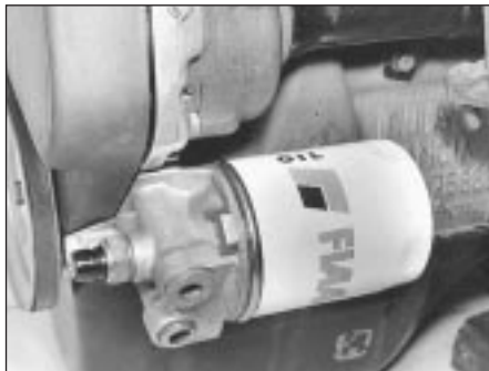
5D.29 Oil filter cartridge and mounting base
