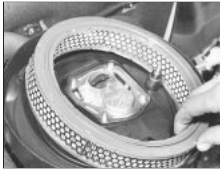
9A.8B Circular type air cleaner element
