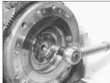
5D.14 Tightening a flywheel bolt
