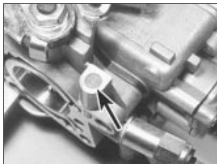
9B.8 Weber 32 TLF 4/250 carburettor mixture screw location under tamperproof plug (arrowed)
