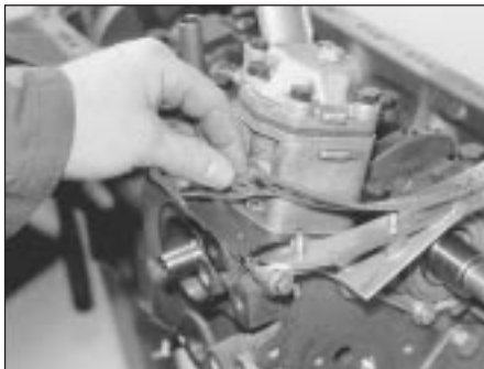
7B.166A Locate the new gasket . . .
