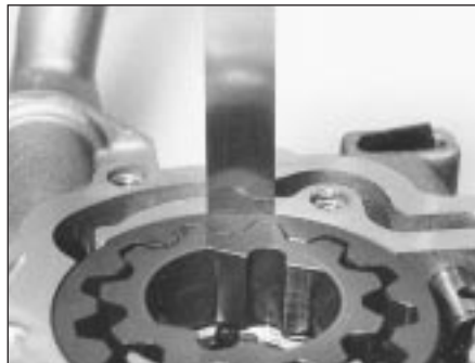
5B.74A Checking the oil pump gear-to-housing clearance
