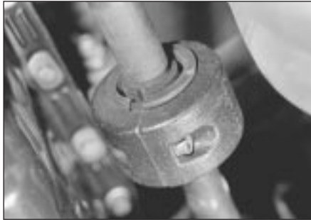
13.24 Right-hand driveshaft damper weight
