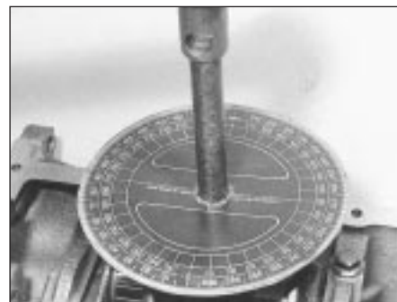
5D.7B Angle-tightening a main bearing cap bolt
