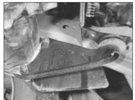
5C.31B Left-hand engine mounting and bracket
