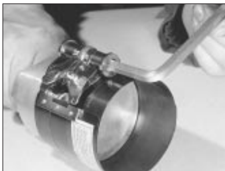
7B.194A Fitting a ring compressor to a piston
