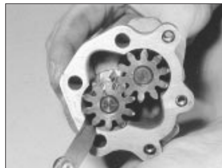
7B.176 Check gear-to-body clearance
