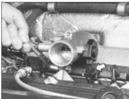
Fig. 13.58 removing the inlet manifold mounting bracket from the cylinder head on the 1372 cc Turbo ie engine (Sec 9E)
