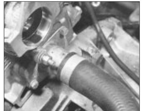
8A.6 The thermostat housing (shown with distributor removal) on the 999 cc engine
