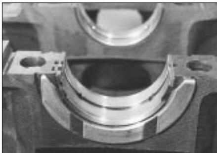
5D.3 Crankshaft thrust washer at centre bearing
