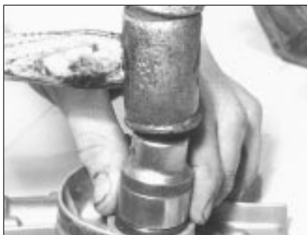
5B.77B Using a socket to fit the new oil pump oil seal
