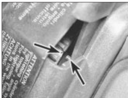
7B.30A Camshaft sprocket timing notch aligned with timing (TDC) pointer in timing case
