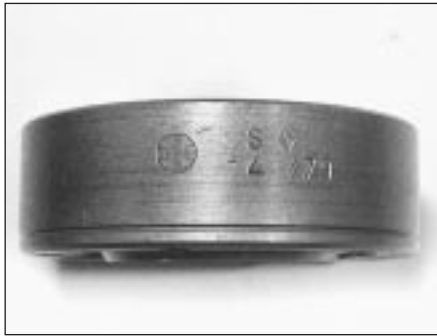
13.21 Outer track reference groove
