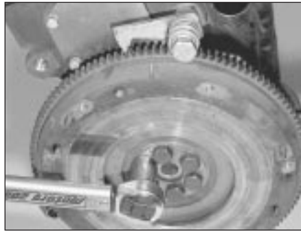
7B.158B . . . tighten the bolts to the specified torque
