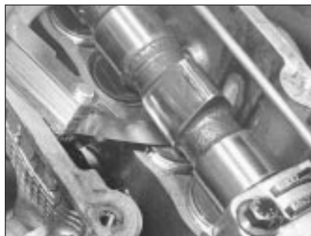
5B.1A Checking a valve clearance
