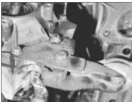
5C.26 Left-hand rear (lower) transmission mounting disconnected
