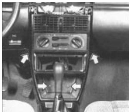
Fig. 13.32 Heater unit facia to main facia retaining screw locations (arrowed) (Sec 8D)
