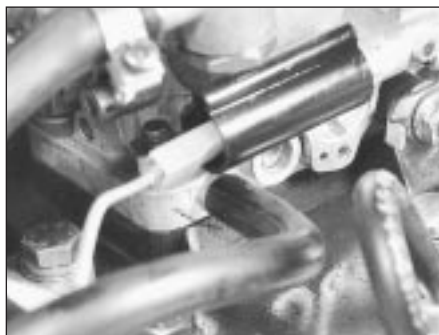
9B.37D Electrical lead to automatic anti-flood device on the Weber 30/32 DMTE carburettor
