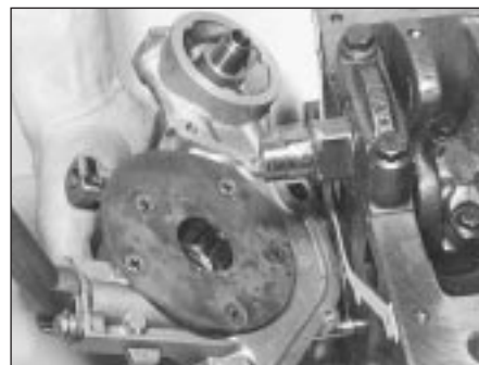
5B.78 Fitting the oil pump
