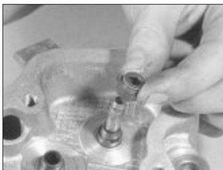
7B.130C . . . locate stem oil seal . . .
