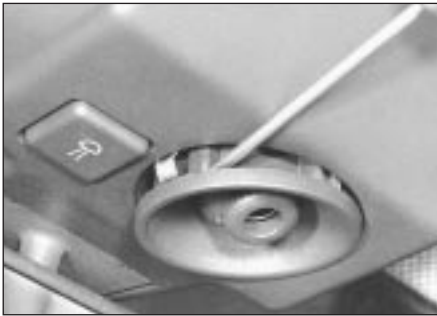
15.80A Prising free the roof-mounted spotlamp
