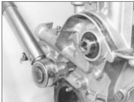
5D.12B Tightening an oil pump bolt
