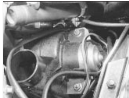
9C.85 Fuel injector cooling fan
