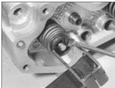
7B.130J Compress spring and refit the split collets
