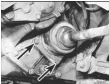
5C.25A Two of the left-hand driveshaft joint gaiter retaining plate screws (arrowed)
