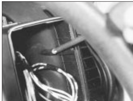
15.55B Facia switch housing inner screw removal on the 1031 cc Turbo ie model
