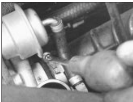
9F.17 Releasing turbocharger air hose clip
