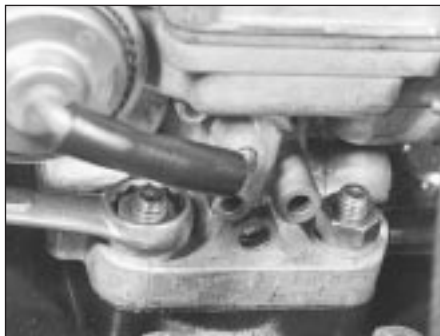
9B.37F Unscrewing a carburettor fixing nut
