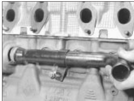
5D.30 Coolant distribution pipe
