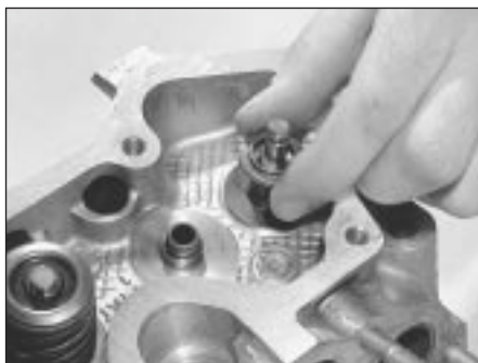
7B130F . . . locate the spring seat . . .
