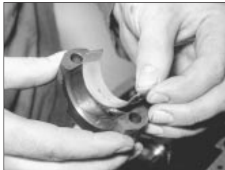
7B.196 . . . and big-end bearing cap . . .
