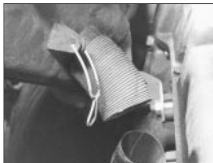
9A.5A Air cleaner hot air intake and lower retaining clip on the 999 cc model
