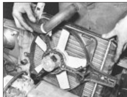
5C.19D Removing the radiator/fan assembly
