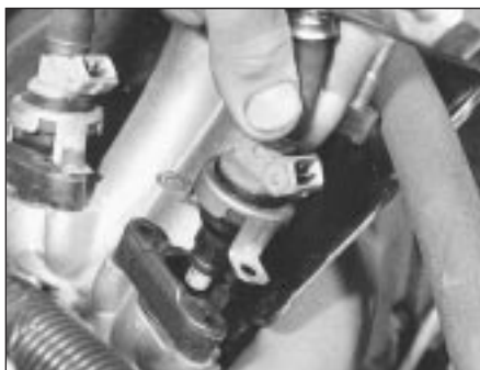
9C.80B Fuel injector removal
