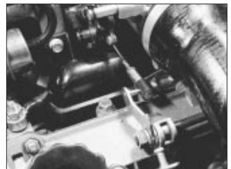
9C.99B Throttle cable (secondary section) and cross-shaft
