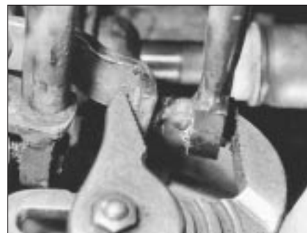
5D.45 Connecting ball socket type gearchange rod
