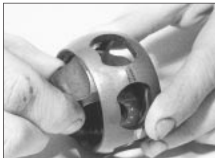
13.19B Separating inner and outer cage members
