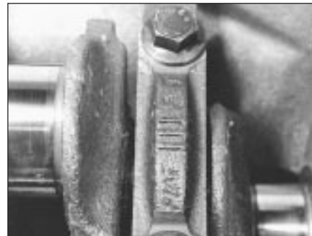
5C.66 Main bearing cap markings
