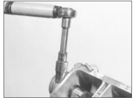
7B.85 Tightening a camshaft housing securing bolt
