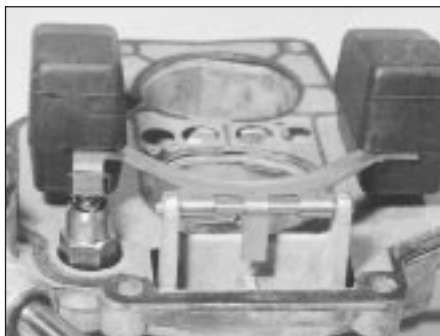
9B.45 Float pivot arrangement and needle valve on the Weber 30/32 DMTE carburettor
