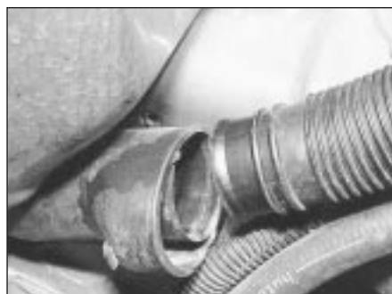
9A.5B Air cleaner cold air intake on the 999 cc model
