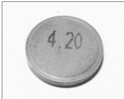
2B.25A Valve clearance shim showing thickness mark
